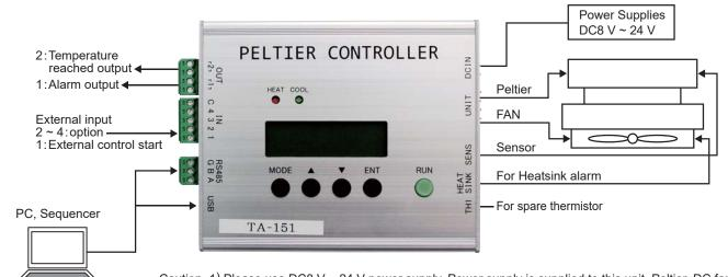
Caution 1) Please use DC8 V ~ 24 V power supply. Power supply is supplied to this unit, Peltier, DC fan. Please use power supply and electric wire with sufficient power capacity. If you add a voltage outside the specified range, it will be damaged.
